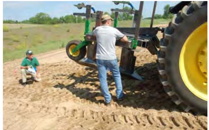
*MSU Professor Alvin Smucker, far left, observes testing of an implement to dig trenches prior to the installation of a polyethylene membrane that will help sandy soils retain water. (above) Research on the subsurface water retention system is funded through a grant from NRCS.*
